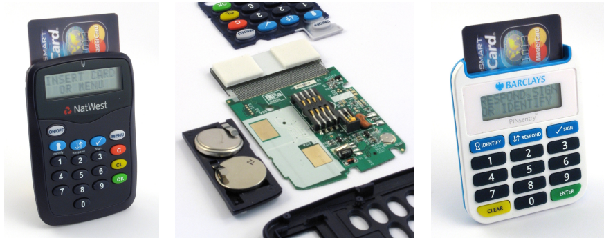
Fig. 1. NatWest and Barclays issued CAP readers on the left and right, respectively. An opened NatWest CAP is shown in the centre. These readers are given to bank customers for free.
