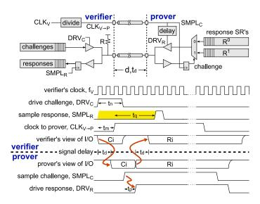
The distance resolution we can achieve is defined by the operating frequency of the verifier and so should have a fast clock, whereas the prover can operate at low frequencies and use delay lines to derive critical signals. We have tested the system with various transmission lengths and confirmed that it is indeed able to detect small additions to the signal transmission distance.
